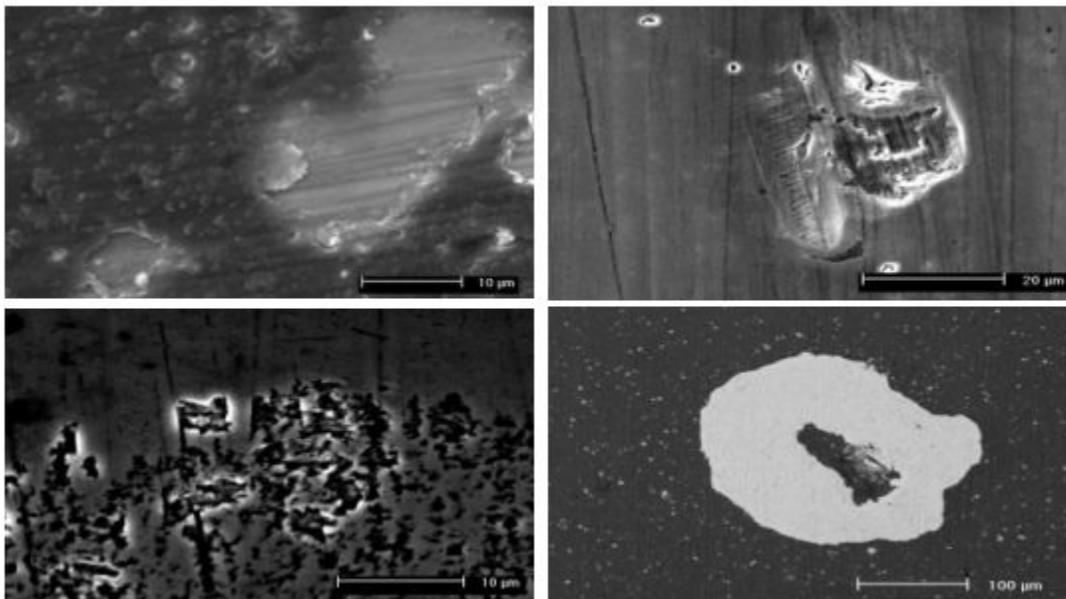
Fig 4 – (a) Localised exfoliation of CotI (after 3 hrs), (b) Polishing, microcracking and tearing of CotIII (after 150 hrs), (c) Polishing and micro-pitting of CotIII (after 150 hrs) and (d) Delamination of CotII (after 15 hrs)
